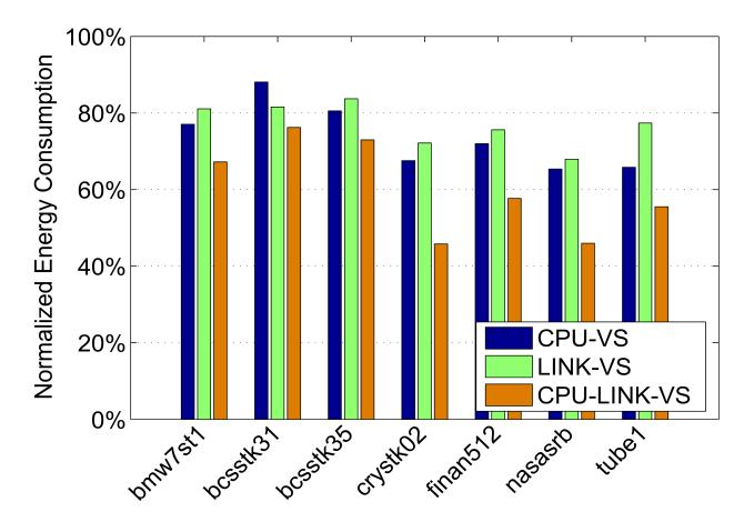
Average Savings: CPU-VS (27%), LINK-VS (23%), CPU-LINK-VS (40%)
