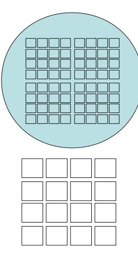
·Manufacturing is imperfect ·Die for 4 chips@ 16 cores • Top fast, high leak · Bottom slow, low leak Variations within chip ·Reorganize computations to model variations ·Schedule and load balance for performance and energy ·Algorithms/software will have to model these variations
