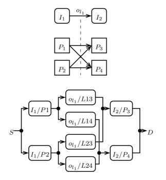
Figure 4: A mapping of two intervals  $(I_1 \text{ and } I_2)$  on four processors  $(P_1 \text{ to } P_4)$  and its RBD which has no particular form.
