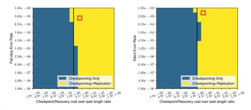
Figure 7: Impact of checkpoint/recovery cost and error rates on the usage of checkpointing and replication. Total sequential work is fixed to 10,000s and is distributed uniformly among n = 20 tasks (i.e.,  $T_1 = T_2 = \cdots = T_{20} = 500$ s). Each color shows the presence of checkpoints and/or replicas in the optimal solution.
