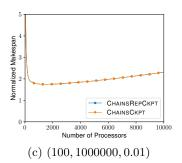
Figure 5: Comparison of the ChainsCkpt and ChainsRepCkpt strategies for different numbers of processors, with different model parameter values for the checkpointing cost  $(a_i, b_i, c_i)$ .
