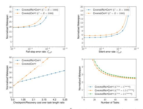
Figure 10: Impact of fail-stop error rate  $\lambda_{ind}^F p$  (left), checkpoint cost (middle) and ratio  $\alpha$  between the checkpointing cost for replicated task  $C_i^{rep}$  over non-replicated tasks  $C_i^{norep}$  (right) for the Uniform distribution.
