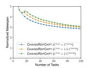
Figure 4: Impact of fail-stop error rate  $\lambda_{ind}^F p$  (left), checkpoint cost (middle), and ratio  $\alpha$  between the checkpointing cost for replicated task  $C_i^{rep}$  over non-replicated tasks  $C_i^{norep}$  (right).
