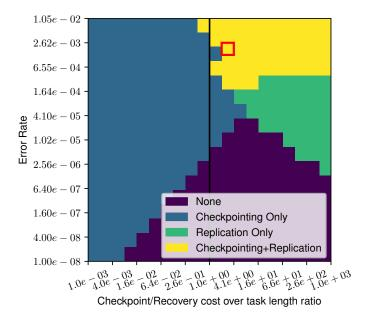
Figure 1: Impact of checkpoint/recovery cost and error rate on the usage of checkpointing and replication. Total work is fixed to 10,000s and is distributed uniformly among n=20 tasks (i.e.,  $T_1=T_2=\cdots=T_{20}=500s$ ). Each color shows the presence of checkpoints and/or replicas in the optimal solution. Results corresponding to the case highlighted with a red square are presented in Figure 2.
