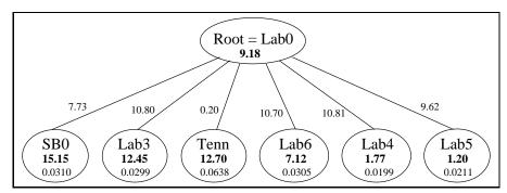
Figure 3. Testbed Fork Graph: Computation Rate Order. Here the leaf nodes are arranged in non-increasing order of computation rate, as used by the CompRate scheduling algorithm.
