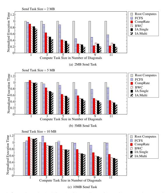
Figure 5. Comparison of scheduling algorithms. To provide a wide range of computation-to-communication ratios, we use task send sizes of (a) 2MB, (b) 5MB, and (c) 10MB. Additionally, compute task sizes varied from 1 to 11 diagonals. The normalized execution time is shown on the y-axis, where each bar represents an execution time normalized to the time of RootComputes.
