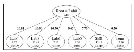
Figure 4. Example Testbed Fork Graph: Maximum Transfer Rate Order. Here the leaf nodes are arranged in non-increasing order of maximum transfer rate, as used by the BWC scheduling algorithm.
