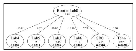
Figure 2. Testbed Fork Graph: Interference Aware Order. Within each node, we list the computation rate in diagonals/sec, and (for child i) its interference rate  $I_s^{root}(i)$  on the root. Each edge shows the transfer rate in MB/sec. Here the leaf nodes are arranged in non-decreasing order of the interference rates. This is the priority of child nodes used by the Interference Aware scheduling algorithms.
