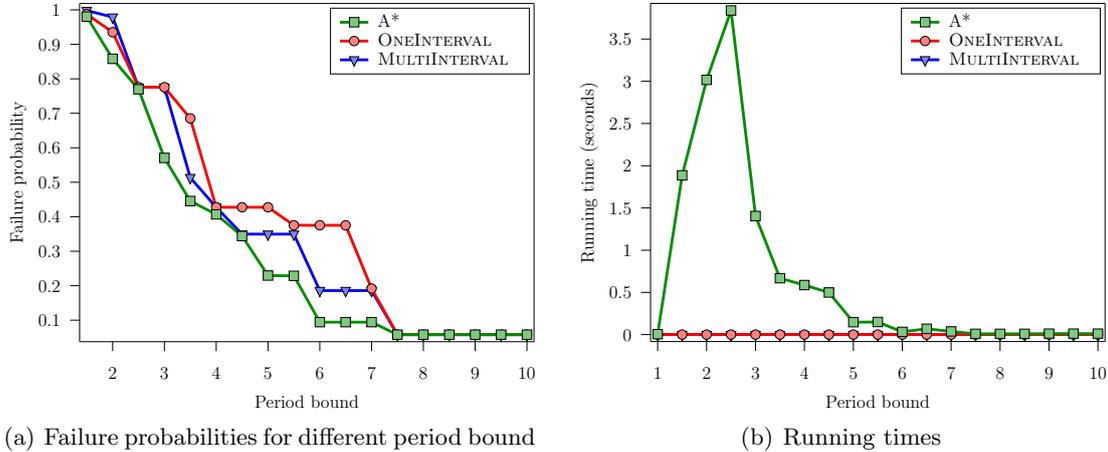
(a) Failure probabilities for different period bound
