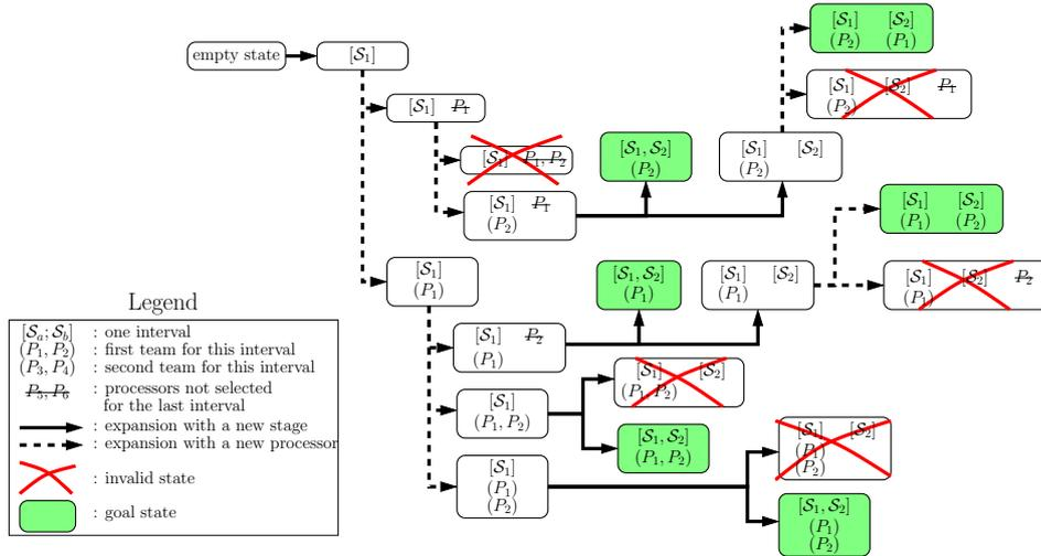
Figure 2: Complete state tree for two-stage application mapped on two processors. E.g., state at bottom right corner is made of a single interval  $[S_1, S_2]$  and two teams with one processor each:  $(P_1)$  and  $(P_2)$ .
