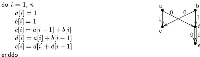
Fig. 12. Original code and its dependence graph.
