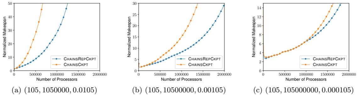
Figure 11: Comparison of the CHAINSCKPT and CHAINSREPCKPT strategies for different numbers of processors, with different model parameter values for the checkpointing cost  $(a_i, b_i, c_i)$ .
