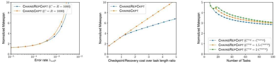
Figure 4: Impact of fail-stop error rate  $\lambda_{ind}^F p$  (left), checkpoint cost (middle), and ratio  $\alpha$  between the checkpointing cost for replicated task  $C_i^{rep}$  over non-replicated tasks  $C_i^{norep}$  (right).
