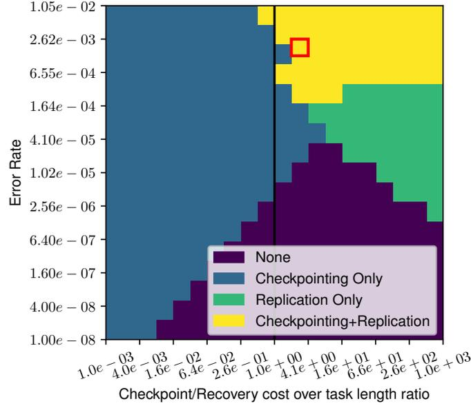
Figure 1: Impact of checkpoint/recovery cost and error rate on the usage of checkpointing and replication. Total work is fixed to 10,000s and is distributed uniformly among  $n = 20$  tasks (i.e.,  $T_1 = T_2 = \dots = T_{20} = 500$ s). Each color shows the presence of checkpoints and/or replicas in the optimal solution. Results corresponding to the case highlighted with a red square are presented in Figure 2.
