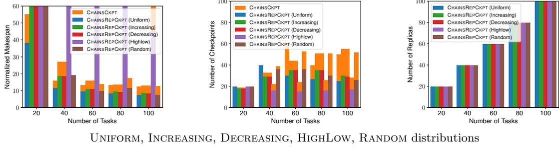
Figure 9: Comparison of the CHAINSCKPT and CHAINSREPCKPT strategies for different numbers of tasks: impact on the makespan (left), number of checkpoints (middle) and number of replicas (right) with a fail-stop error rate of  $\lambda_{ind}^F p = 1.28e-3$ , a silent error rate of  $\lambda_{ind}^S p = 5.48e-3$  and a constant checkpointing/recovery cost  $C_i^{norep} = C_i^{rep} = 1000s$ .
