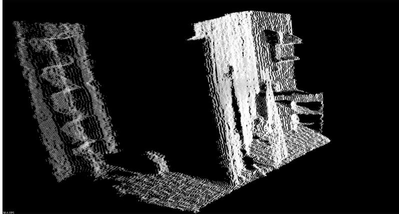
Figure 8: 3D point cloud created from the depth map of the Kinect
