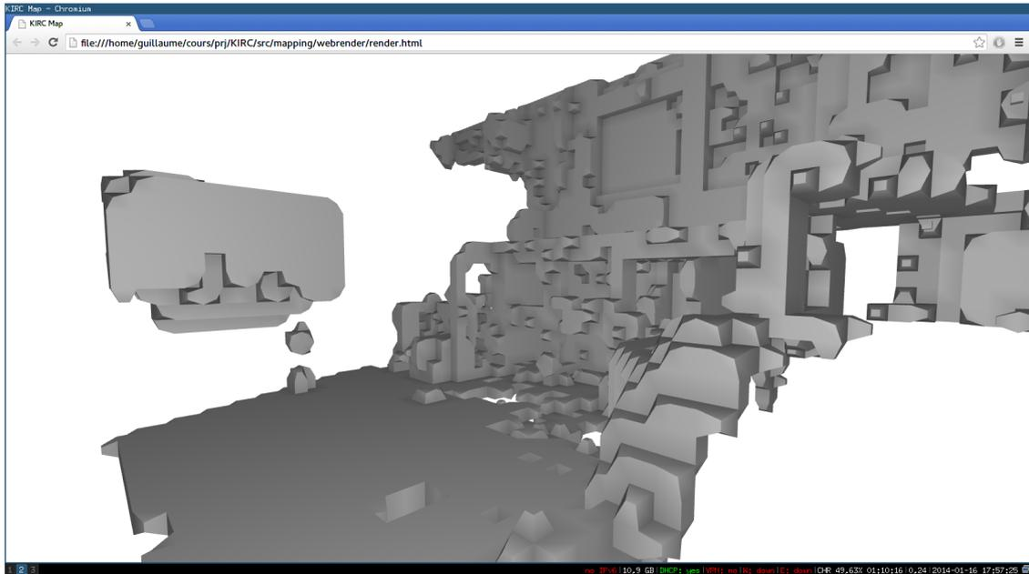
Figure 11: Image of a room with shelves with the Negative density method and a fixed kinect
