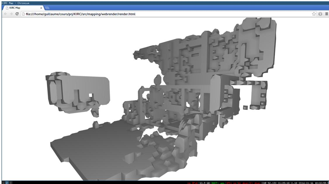
Figure 10: Image of a room with shelves with the Basic density method and a fixed Kinect
