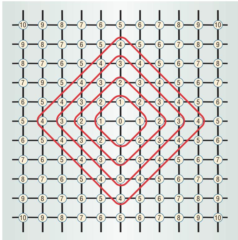
**Figure 1. Load distribution flow in a 2D network. The load originates at node 0 and propagates throughout the mesh in a diamond-shaped pattern. (Reprinted with permission from the Poznan University of Technology.)**
