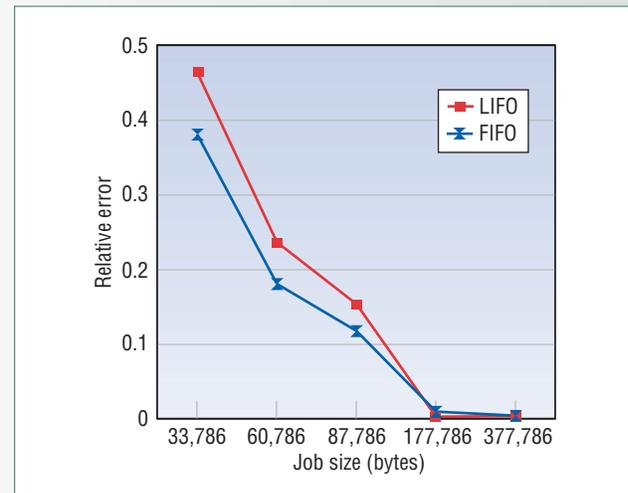
**Figure B. Difference between modeled predictions and measured values for a join-type relational database operation. Divisible load theory's accuracy increases with job size. (Reprinted with permission from: M. Drozdowski and P. Wolniewicz, "Experiments with Scheduling Divisible Tasks in Clusters of Workstations," LNCS 1900, Springer Verlag, 2000, p. 318.)**
