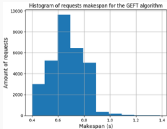
Figure 15: Makespan for the GEFT algorithm.
